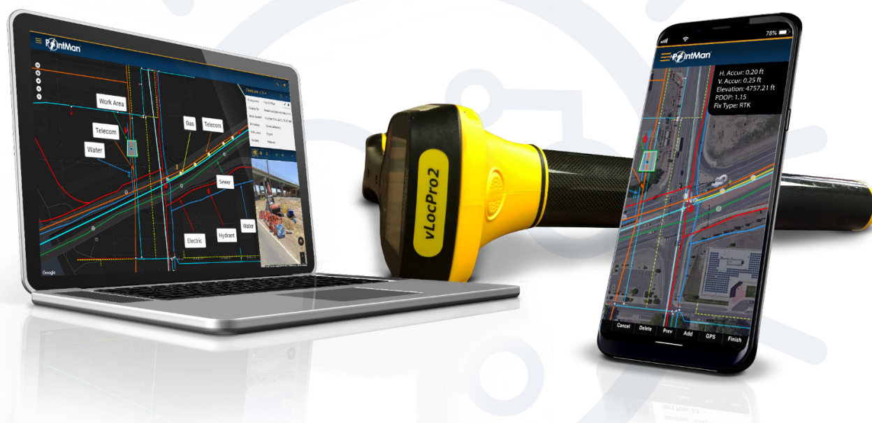
Figure 1 - Laptop displaying PointMan Pro (left), Vivax EM Locate tool (middle), Android phone displaying PointMan application
